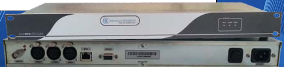
Example of transporting two different radio programs (in MPX format), simultaneously to multiple FM broadcasting sites
